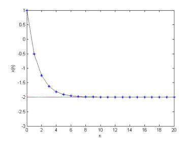
Figure 2.3: The Stability of  $\bar{x} = -2$  of  $x(n+1) = \frac{1}{2}x(n) - 1$
